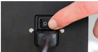
5) Plug in the power cable and turn on the power switch at the back of the machine.
