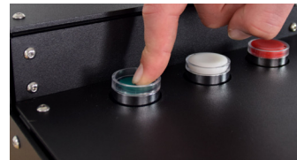
7) Press the green button down for one second to start the machine.
