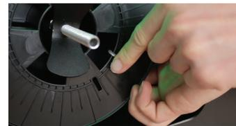
**15)** Guide the filament through the spool (inner hole).
