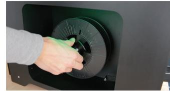
**7)** Place spool holder with spool on the spooling axis.
