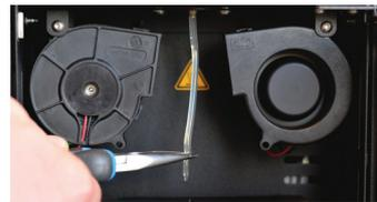
**10)** When the filament is extruding, wait until about 20cm is out of the nozzle.
