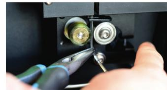
**11)** Open the puller clamp, then pull the soft filament through the Optical diameter sensor and puller.
