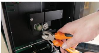
**13)** Cut the filament when the set size is reached and start spooling.
