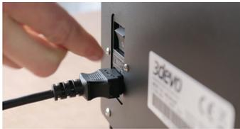
**1)** Plug in the power cord and turn on the power switch at the back of the filament maker.
