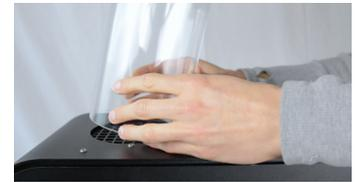
**4)** Unwrap the hopper tube and place it on top of the extruder hopper.
