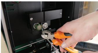
**13)** Cut the filament when the set size is reached and start spooling.
