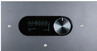
**9)** Main screen will indicate that the system is 'Heating'. Wait about 10 minutes and the extrusion process will start automatically.
