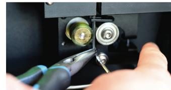
**11)** Open the puller clamp, then pull the soft filament through the Optical diameter sensor and puller.
