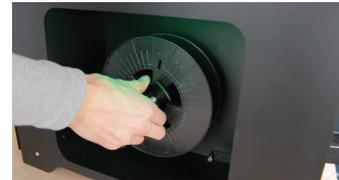
**7)** Place spool holder with spool on the spooling axis.
