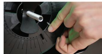
**15)** Guide the filament through the spool (inner hole).
