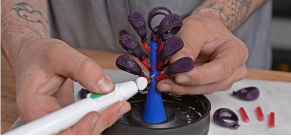
A [wax heat pen](#) makes it easier to join resin patterns to the wax sprue tree.
