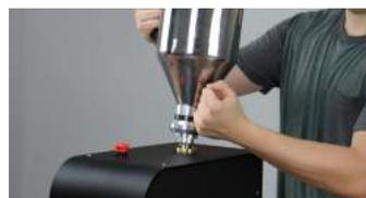
11) Wait until the program is finished. When finished, loosen the quick release nut. (Be careful for the hot surfaces)
