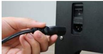
1) Plug in the power cable and turn on the power switch on the back of the machine.
