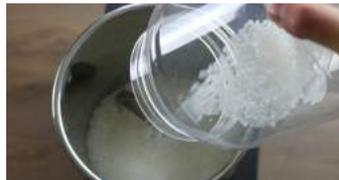
6) Fill the hopper with your plastic granules, powder or regrind and put the lid on the hopper.
