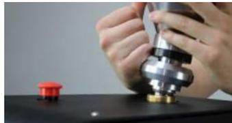
2) Place hopper on the dryer and make sure the rotational coupling on the bottom of the hopper is engaged.
