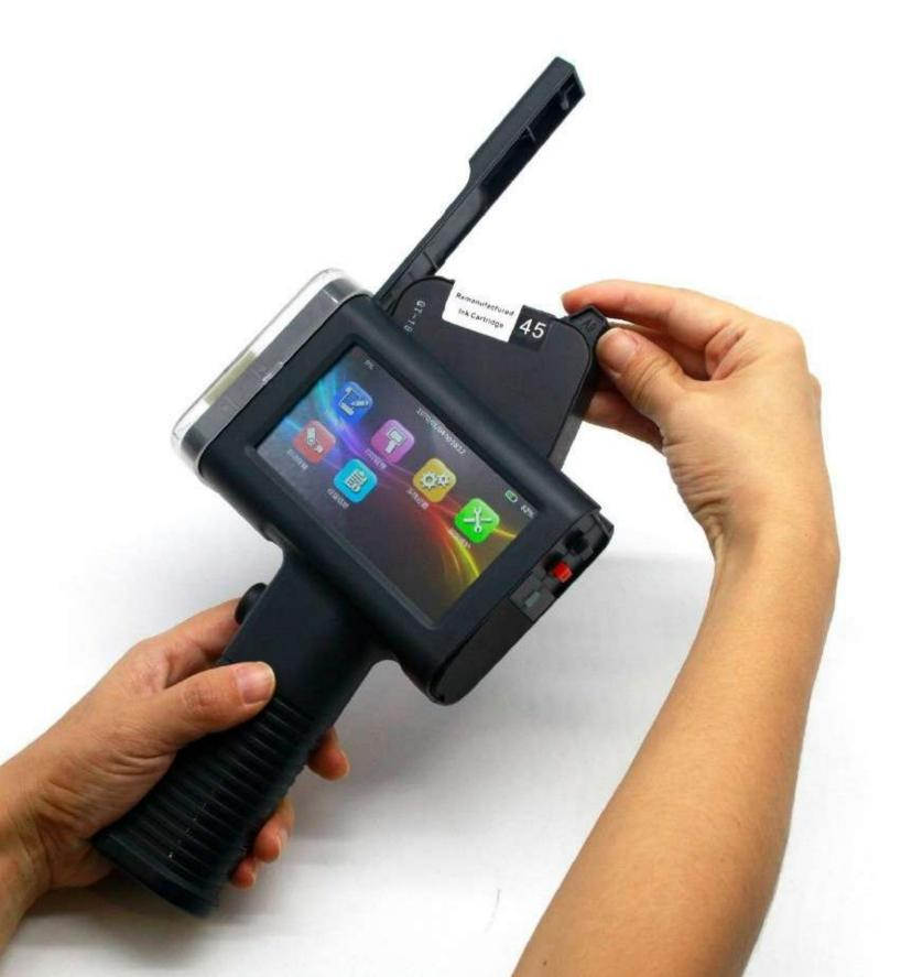
The unique hardware protection scheme of Ekoprint can disassemble and assemble ink cartridges electrically.
